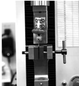
(c) Copper collar retention force: IUD in clamp
