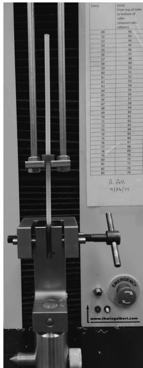
(b) Flange force test set-up
