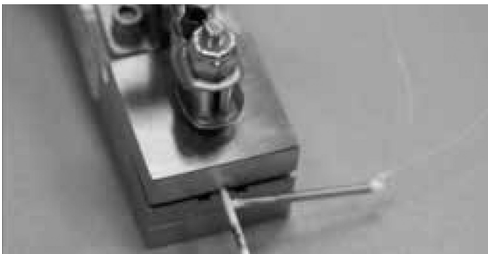
(c) Copper collar retention force: IUD in clamp
